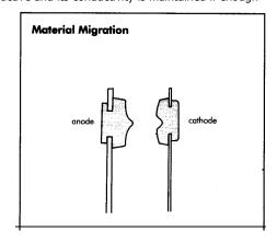
wear and migration from cathode to anode causing rapid wear. (DC circuits only) Craters and cones eventually lead to failure due to mechanical interlocking and the reduced air gap.
