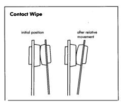
invariably covered with thin layers of oxides, sulphides and other compounds formed by gas molecule absorbtion. Particles created by wear also appear soon after use. Mechanical cleaning can be designed in to allow contact surfaces to wipe
